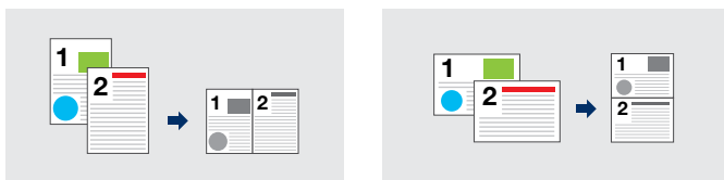
2IN1: Copies two pages on a sheet of paper in portrait or landscape orientation.
